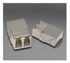
Razor series optical fiber transceivers consist of optoelectronic transmitter and receiver functions integrated into a printed circuit board mounted Duplex LC compliant receptacle connector. The optical transmitters are 850 Nm VCSEL lasers. The transmitter input lines are driven with differential CML signals applied to the transmitter (TX+ and TX-) lines. Dual loop, temperature compensated, VCSEL drivers convert the transmitter input signals to suitable VCSEL bias and modulation currents.
