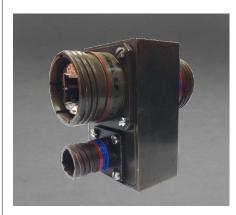
Saturn series Fast Ethernet media converters consist of optoelectronic transmitter and receiver functions integrated along with the 10/100Base-TX Ethernet electrical to 100Base-FX Ethernet optical media conversion circuitry into an environmentally sealed unit.
